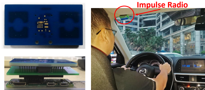
Fig. 19. COTS impulse radio used in V 2 iFi and radio setup inside the vehicle.
